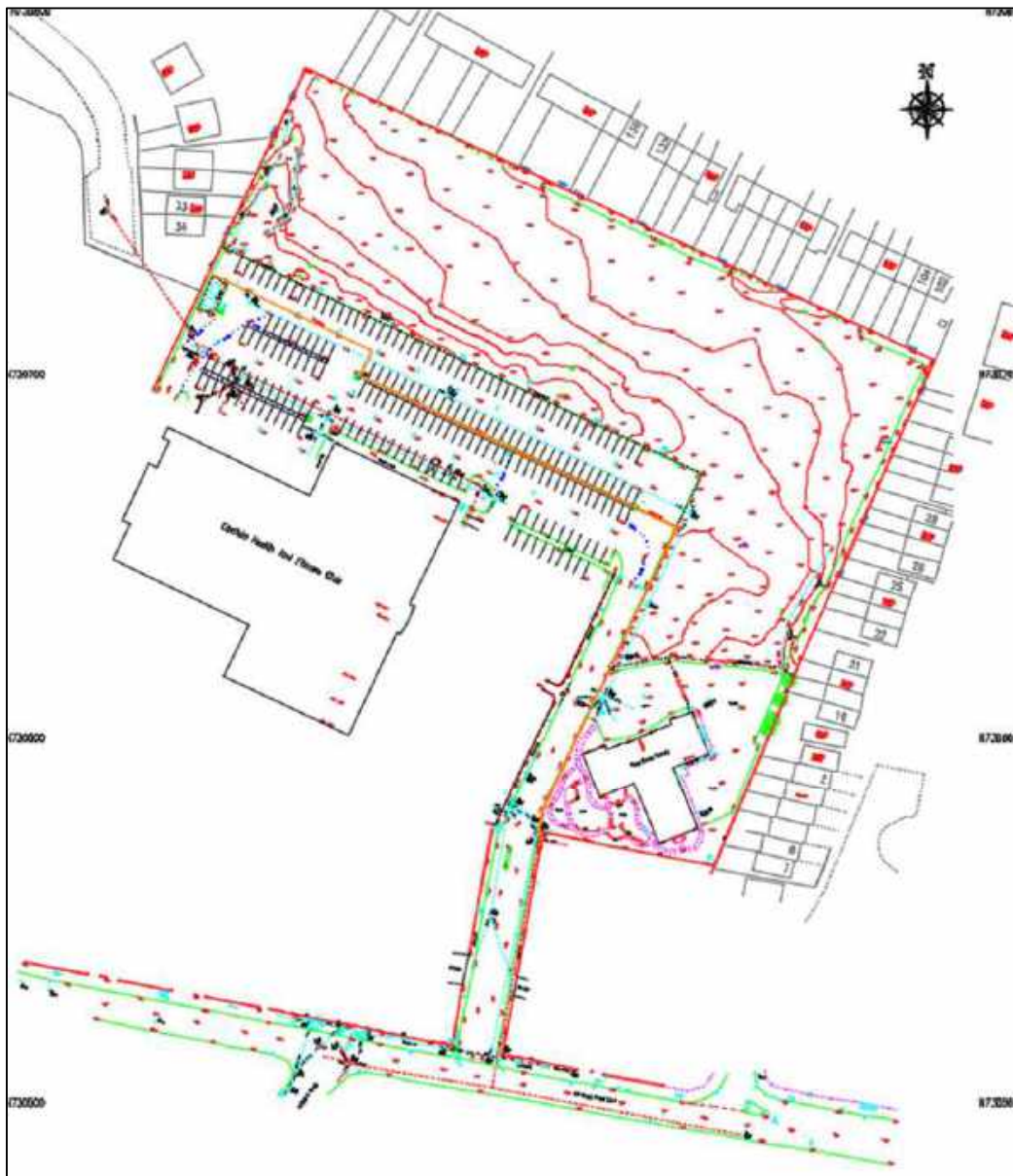
Figure 2-1: PCA Topographical Survey Extent
