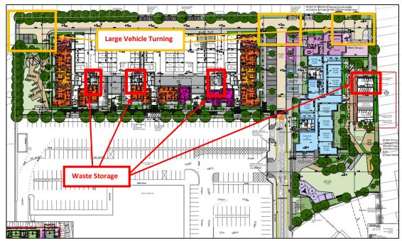
Figure 3.1 Extract of BKD Architects Drawing (Waste Storage Areas) and Large Vehicle Turning Areas
