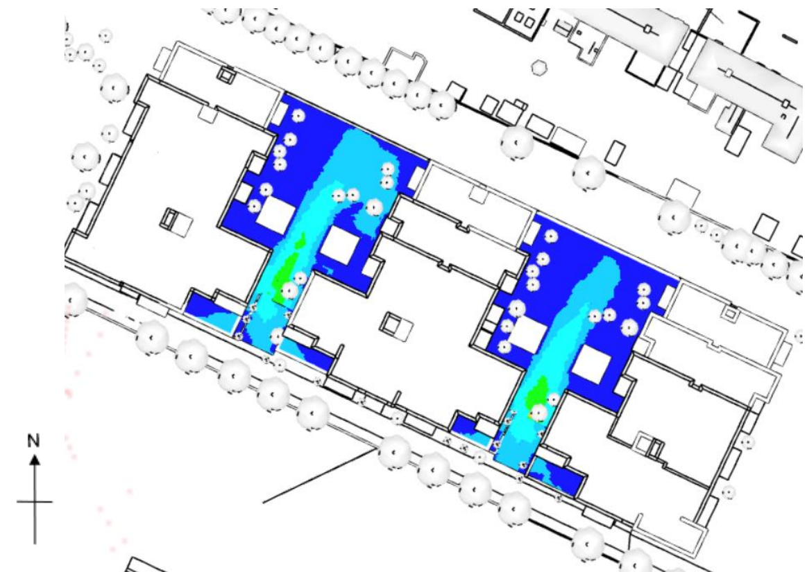
Fig. 4.3.2 – Lawson Criteria results at 1.5m above podiums including proposed landscaping.
